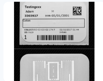
Integral RFID + barcode label
