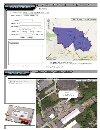
● A Web-based Fleet Central Application enables authorized users to securely access real-time information from specific geographic regions. Data are transmitted from remote assets by the Quake Global Q9612 modem (bottom inset).
