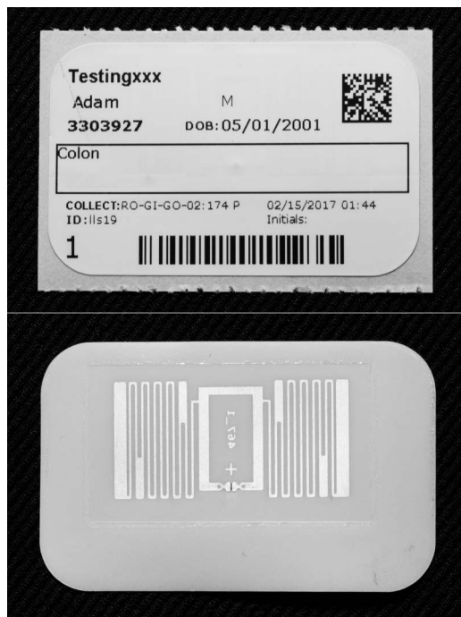
Figure 1. Sample radio-frequency identification (RFID) tag. Integrated ultrahigh-frequency RFID tag, 2D bar code, and 1D bar code for specimen identification (front and reverse).
