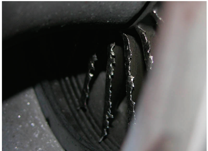
Figure 1: Turbine blade damage caused by Foreign Object Debris (FOD)
